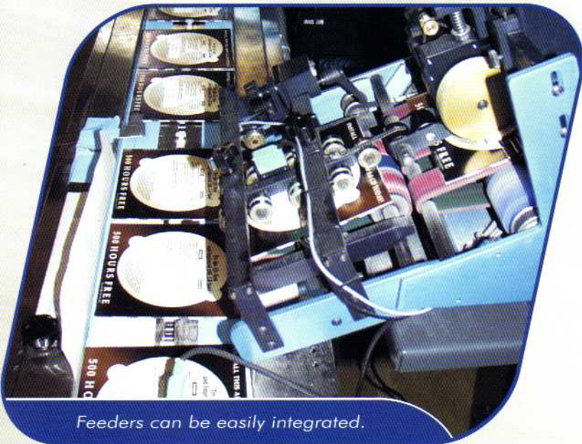
Belts control the material all the way through the feeder.
