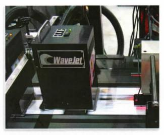
DOD Piezo Print Heads produce high-resolution images and can accomodate a wide variety of different inks.
